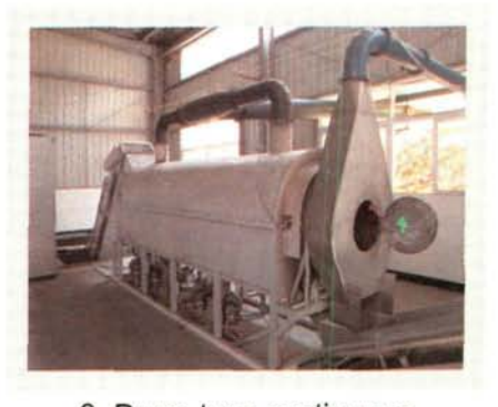
9. Drum-type continuous de-enzyming machine
